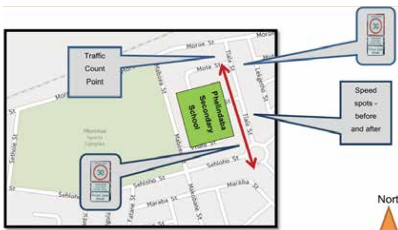
Figure 6. Installed two-speed limit boards on each side of entry of the school zone at Maboea Street
